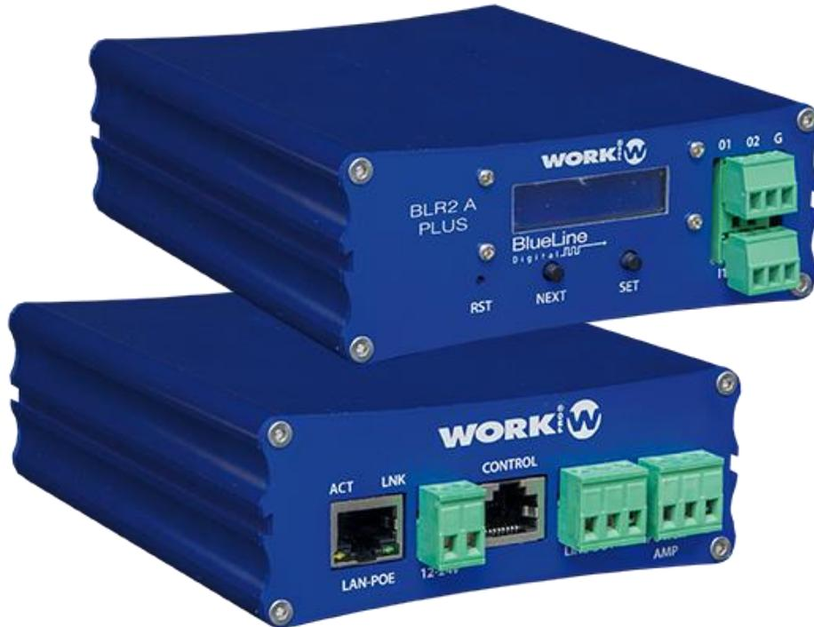
The BLR2 A PLUS MKII is an audio over IP receiver, that can extract one of the channels transmitted by the BlueLine MKII senders with a built-in amplifier.
